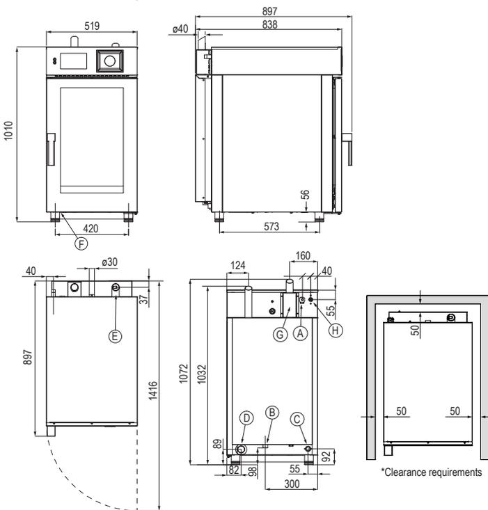
**Heat Source:** 500mm clearance from an external heat source is required in order to protect the oven control components. For clearances under 500mm, it is mandatory for Stoddart heat shields to be fitted while still maintaining a minimum clearance of 50mm to allow access to the unit. Failure to adhere to minimum clearances may void the oven warranty or add service costs due to lack of access.
