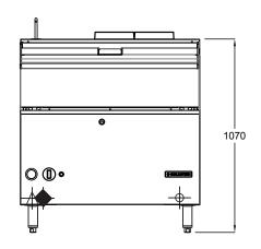
3/4" BSP Gas Inlet 10 AMP/230V Plug with 3m Lead Cable − 1/2" Quick Connect Water Inlet
