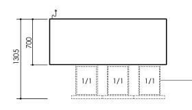
Fully extendable drawers suitable for 100mm deep gastronorm pans. The pan top lip maximum height should be no more than 5mm.
