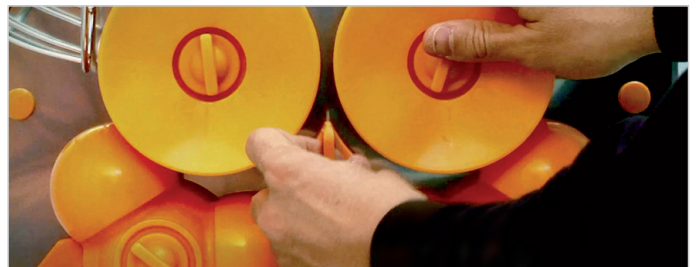
16. Put on the knife. Push until it clicks into place with a "click".
