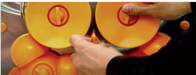
5. Extract the knife by pulling it towards you. CAUTION! The blade is very sharp, be careful not to cut yourself.
